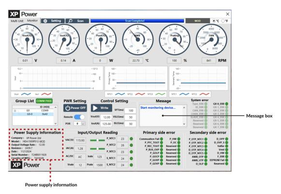
▶ 2.5 - Click Power ON to switch ON the power supply or devices
